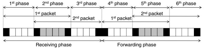
Fig. 2. Timing diagram of the 6-phase relaying used in the analysis. The gray shaded areas indicate the portions of the packets (in terms of symbols) that are overlapped. The black shaded areas indicate packet preambles and postambles that are used for channel estimation.
