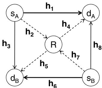
Fig. 1. Analog network coding of independent signal transmissions with the help of a relay. The packet transmissions are received intentionally (thick solid lines) and unintentionally (narrow solid lines) at the destinations. Signal reception and forwarding at the relay is indicated with dashed lines.
