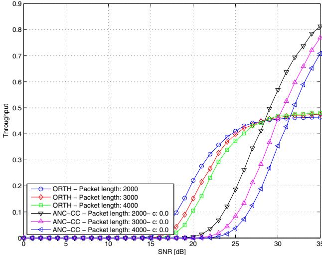
Fig. 5. Throughput comparison for varying packet lengths
