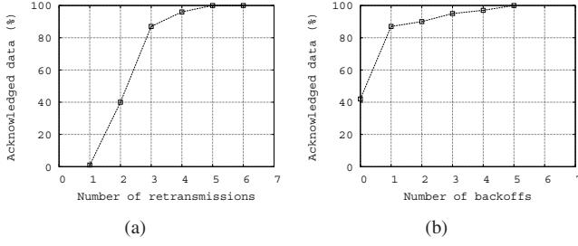
Fig. 6. Throughput vs. the allowed number of retransmissions and backoffs.
