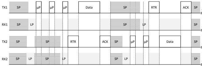
Fig. 3. Representative packet transmission procedure between two nodes.
