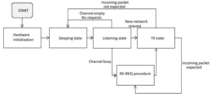
Fig. 2. Generic view of the state machine and interactions with the receiver interrupt service routine (RX\_IREQ).
