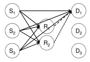
Fig. 1. The basic network scenario considered in this paper is cooperative unicast video transmission with the help of relay nodes  $R_1$  and  $R_2$ . Different line styles indicate transmission in a different time slot.
