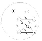
Fig. 1. Ad hop network topology that demonstrates physical layer network coding with cooperative relaying through node  $N_3$ . The solid lines indicate the concurrent broadcasting of packets from  $N_1$  and  $N_4$ , while the dashed lines indicate the forwarded mixed packet from  $N_3$ .
