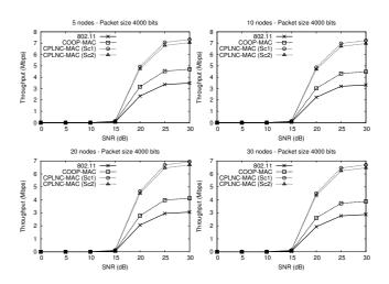
Fig. 4. Simulation results of the aggregate network throughput for different channel conditions and different number of nodes. Packet size of 4000 bits is used.
