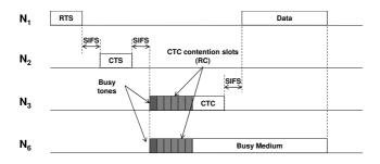
Fig. 3. Distributed optimal relay selection based on prioritization.
