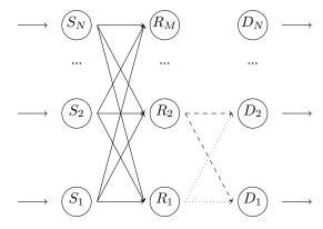
Fig. 1. System model for the cooperative scheme that employs distributed *Space-Time Superimposed Symbol Coding (STSSC)*. Different line styles indicate transmissions in different time slots. For the channels with the dashed lines not all connections are depicted to avoid clogging the figure.
