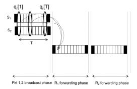
Fig. 2. Behavior of STSSC in the time domain. With STSSC the signal that is forwarded during one symbol slot is a linear combination (dashed lines) of all the superimposed symbols  $q_r$  that were received during the broadcast phase (grey ellipses).
