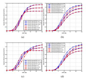
Fig. 2. Spectral efficiency results: a) average channel gain for all channels is 1, b)  $\mathbb{E}[|h_{1,2}|^2] = 0.1$ , c)  $\mathbb{E}[|h_{2,1}|^2] = 0.1$ , d)  $\mathbb{E}[|h_{1,2}|^2] = \mathbb{E}[|h_{2,1}|^2] = 0.1$ .
