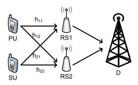
Fig. 1. The cognitive wireless cooperative network model we consider in this paper consists of two users and two relays in an uplink transmission scenario.
