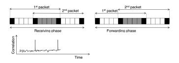
Fig. 3. Collided packets at the receivers and the relay in terms of symbols. Correlation with the preamble spikes when the preambles and postambles of two packets coincide.
