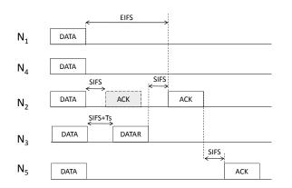
Fig. 2. Timing diagram of the distributed MAC protocol for the topology in Fig. 1. The dark-shaded ACK packet indicates the behavior in a successful direct transmission.
