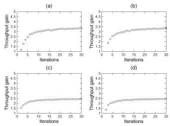
Fig. 10. Total throughput gain in the complete network versus the number of iterations of the cooperative algorithm. The term iterations refers to the number of invocations of the cooperative PHY rate-adaptation algorithm that are executed by a single node. Simulations are presented for different number/ density of wireless nodes. (a) Nodes = 25, degree = 5. (b) Nodes = 50, degree = 3. (c) Nodes = 25, degree = 3. (d) Nodes = 50, degree = 3.
