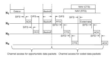
Fig. 3. Channel access with the link-layer network coding protocol.
