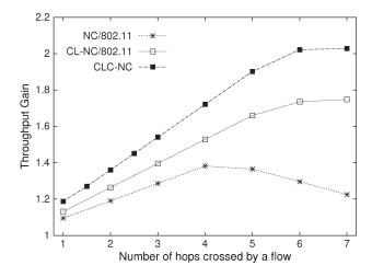
Fig. 7. Throughput gain for a different number of hops crossed by a flow. The percentage of multihop flows is 40%.
