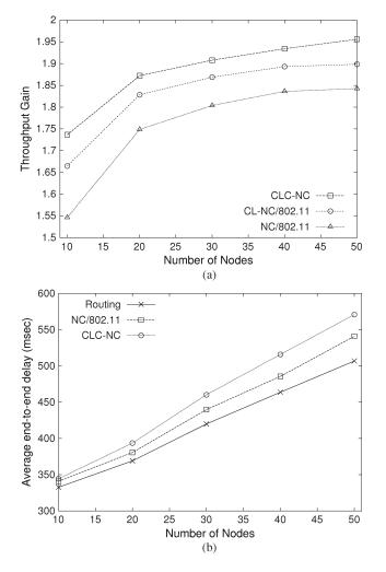
Fig. 6. Simulations results for different number of nodes in the wireless network.
