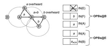
Fig. 2. Operation of single-hop network coding with opportunistic listening enabled. Wireless nodes use the last successfully received packet as an indication of the buffer contents of their neighbors.
