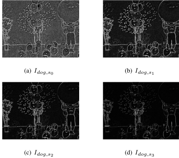
Fig. 2. The different spatial frequency band components I_{dog,s_0} , I_{dog,s_1} , I_{dog,s_2} , I_{dog,s_3} of an given image in Balloons clip, and s_0 = 0 , s_1 = 1 , s_2 = k \cdot s_1 , s_3 = k \cdot s_2 denote the standard deviations of Gaussian response, respectively
