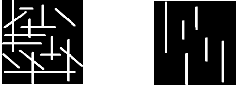
Figure 4: The effect of an Open filter using a vertical 3x9 mask. Only vertical lines with a height of at least 9 and width of at least 3 are preserved.
