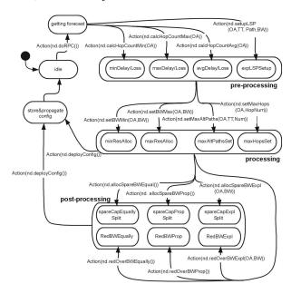
Figure 1: Network Dimensioning module behaviour.
